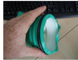
3. Position O ring in top rung of cone.
