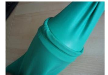
5. Position Sleeve O ring over Glovezon cone and pull tight.
